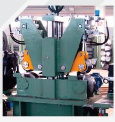
This test is carried out on the entire length of the tubes in order to guarantee the integrity of the hole tube wall.
