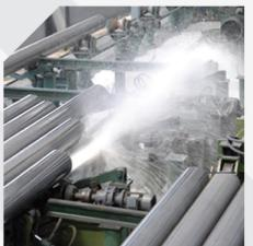
100% Hydro testing is carried out on all pipes and tubes using a high-pressure pump.
